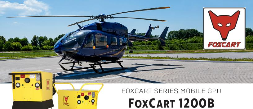
The FoxCart Series 1200 mobile GPU automatically provides plug-head performance IAW ISO 6858 within the limits of ISO 461-1 for output cables up to 20 feet in length when functioning as a maintenance, repair and engine start cart. This 28VDC GPU supports aircraft requiring typical loads up to 600 amps. Engine starting currents up to 1200 amps are provided when operating from its specified 60Hz source and
